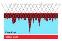
High Performance Polishes by Waxpol bond with the surface's top layer, while filling microroughness to create a smooth & durable protective layer that is reflective, Hydrophobic & easy to clean.
